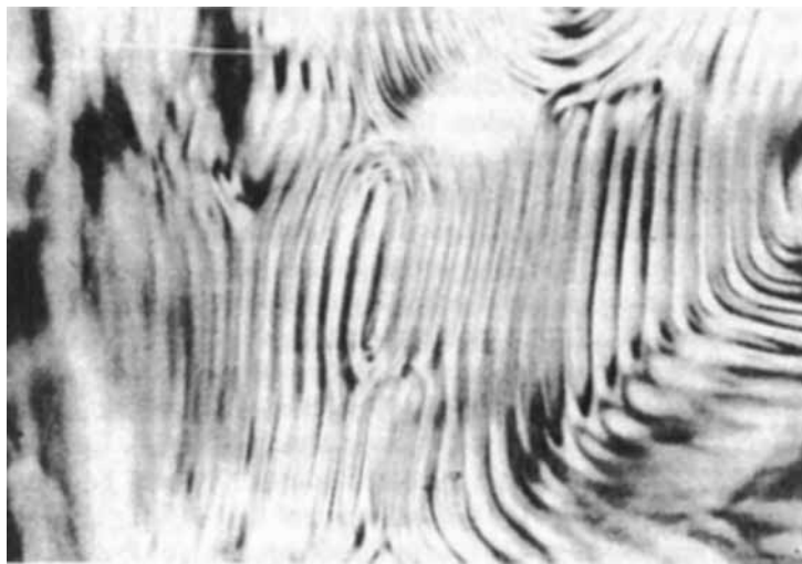
FIGURE 1 Photomicrograph of PBLG/benzene liquid crystal (21.7% wt/v of polymer) in the polarization microscope showing cholesteric texture. The distance between the equispaced retardation lines is one-half the pitch of the cholesteric structure.
